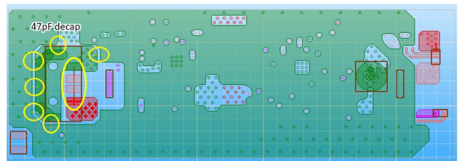
(b) Decoupling capacitor implementation corresponding to Fig. 8 (b)
